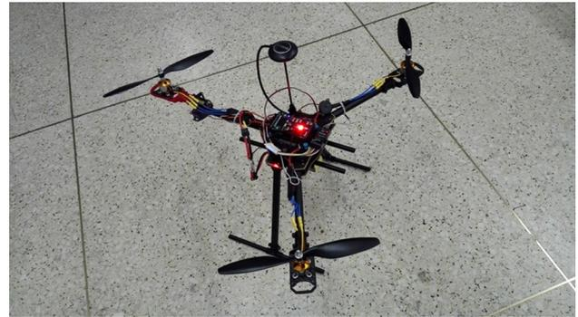
Fig. 1 The Tri-Rotor aircraft
